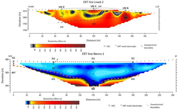
*Figure 4* ERT inversion models with embedded VES 1-D interpretation Up: ERT-2 from "Livadies" pond (RMS=4.6%, 6<sup>th</sup> iteration). Down: ERT-1 from "Nevropolis" pond (RMS=4%, 7<sup>th</sup> iteration).
